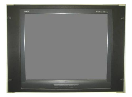
6. Assemble the L-brackets onto the U-Bracket. Adjust the L-bracket so that the monitor screen is centered with respect to the opening of front panel. Also, adjust the L-bracket so that the monitor just touches the backside of the front panel. Lift the monitor on the left side at a slight angle. Insert No. 10 flat washers and 10-32 locknuts onto the left L-brackets. Use a 3/8 socket or
