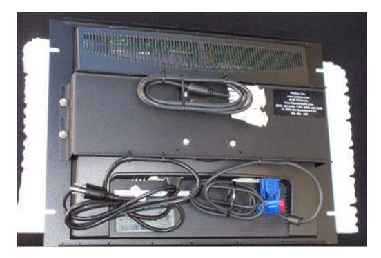
9. The monitor is now assembled. Before mounting it onto a rack, test the rackmount monitor assembly by connecting it to a computer. When done, mount the assembly onto a rack with the four black 10-32 rackmount screws with nylon washers.
