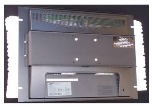
7. Insert a No. 10 washer and a 10-32 locknut onto each stud (two on the right and two on the left). Use a 3/8" socket or crescent wrench to secure the front plate, as shown below:
